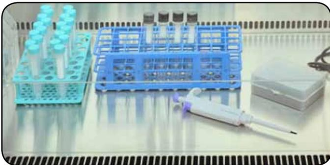
**ULPA filters provide an ISO Class 3 work zone** vs ISO Class 5 of HEPA filters, thus offering substantially better product protection for your precious work.
