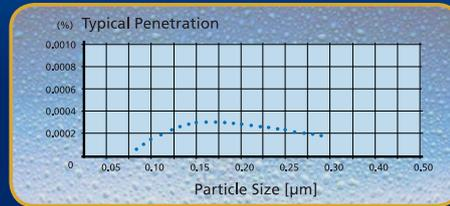
Esco cabinets use ULPA filters (per IEST-RP-CC001.3) / H14 per EN 1822 instead of H13 HEPA filters used on many BSCs in the market.
