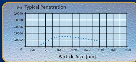
Esco cabinets use high grade H14 filter that offers 99.999% efficiency for particle sizes of 0.1 to 0.3 micron, better than conventional H13 HEPA filters that only offers 99.99 % efficiency at 0.3 micron.
