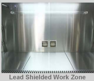
Lead Shielded Work Zone
