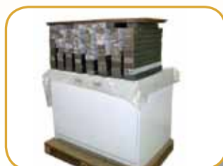
Actual photo during Cabinet Load Testing
