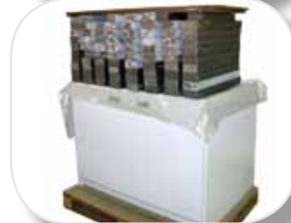
Cabinet Load Test
